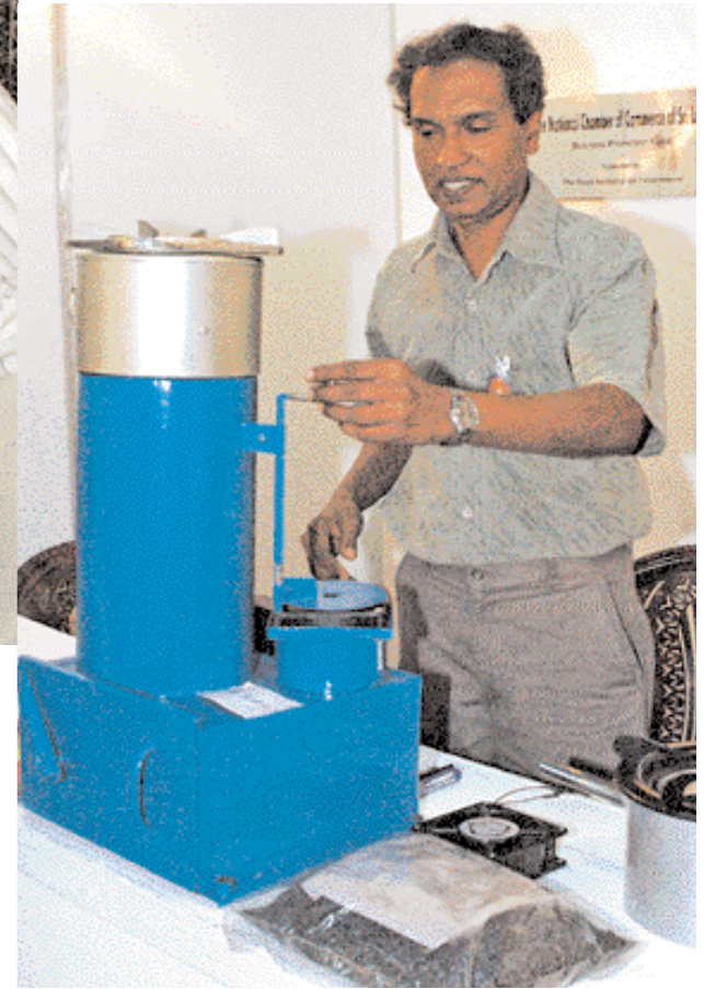
■ This cement block machine designed by Zaearias Joseph produces building material using a soil and cement mixture at low cost
