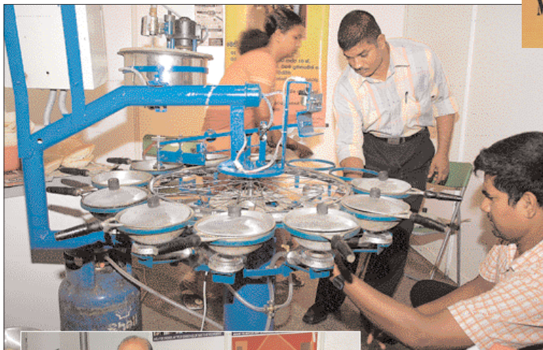
This Hopper Machine invented by Ruhuna University and developed at Industrial Development Board. It could produce 12 hoppers for a minute. This attracted many visitors at the event.
